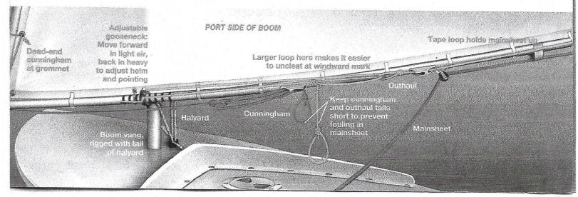
the port side of the boom, far enough forward so that the tails of the lines will not get caught in the mainsheet block, yet still be within reach. Make certain to center the cleats between two clips so that there will be no interference as the clips slide fore and aft with the adjusting of the outhaul and cunningham.
