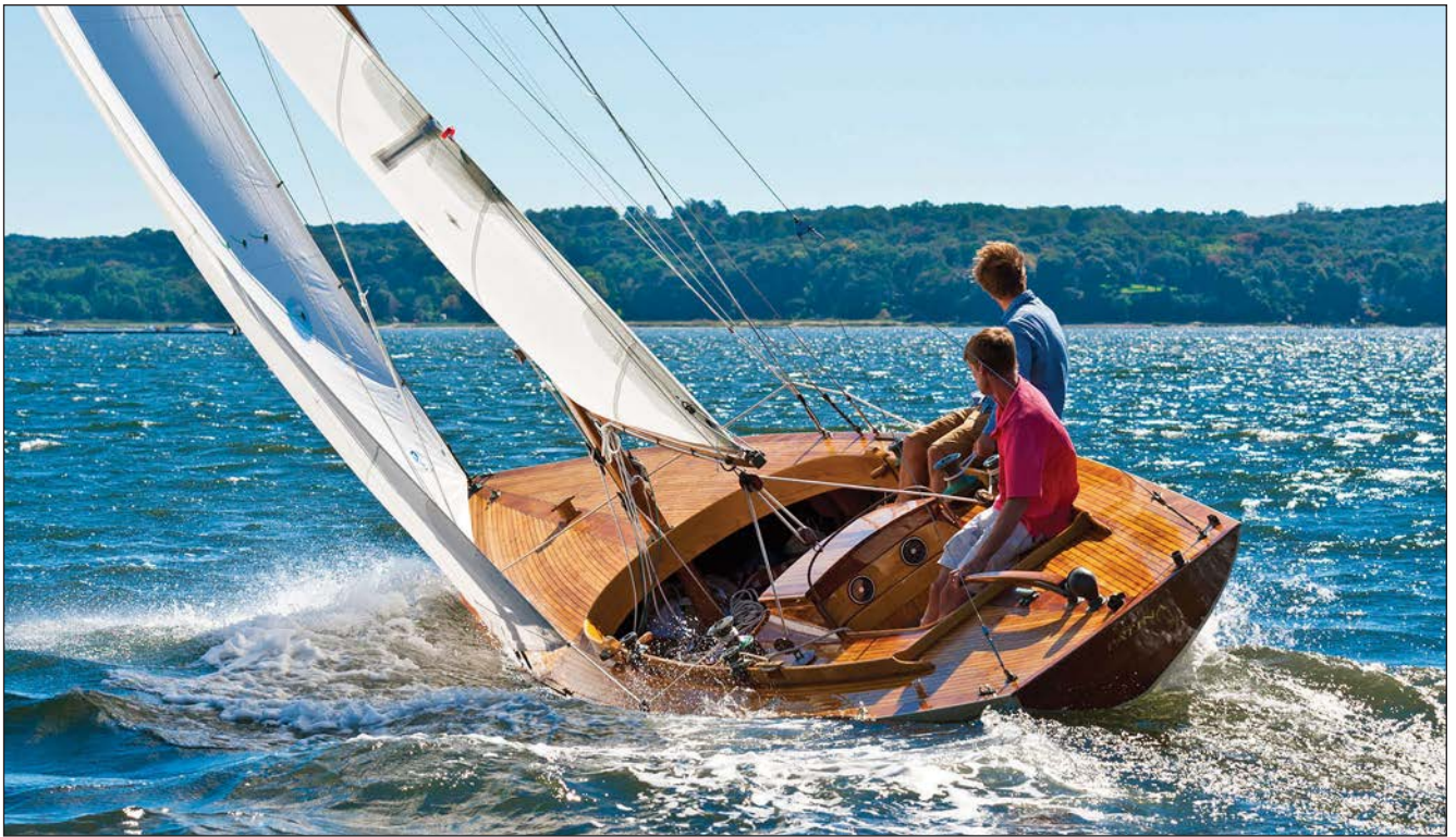
In 2011 at Wooden Boatworks, PATINA, a modified 1956 King's Cruiser sloop designed by Tord Sunden and built in Sweden, received new keelbolts, floor timbers, and a complete cosmetic refurbishing. PATINA had been converted for racing by replacing her cabin trunk with a twin-cockpit layout prior to her arrival at the yard. Wooden Boatworks repowered and rewired PATINA, installed new instruments, and rigged her with new running rigging, bronze deck hardware, and new sails.
